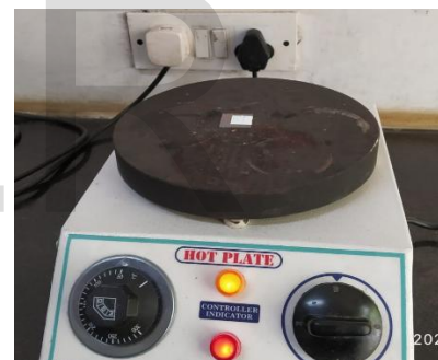
Fig.4 TiO 2 coated glass placed on Hot plate
